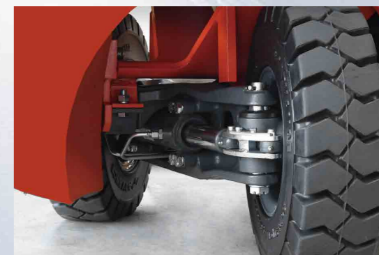
Casting steering bridge
